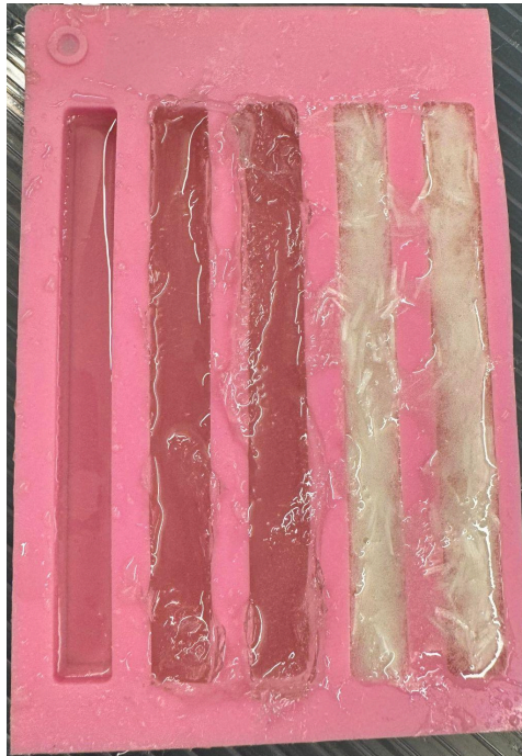
Figure 1: Composite beams in the mold prior to curing.
