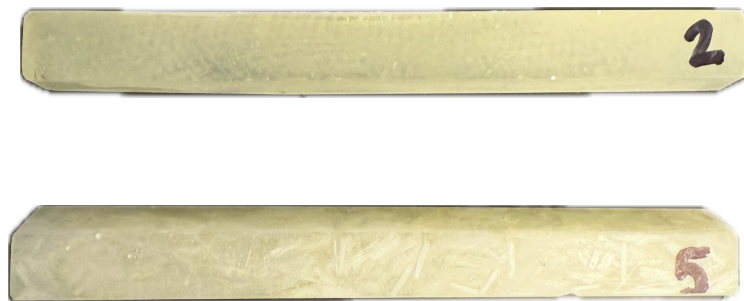
Figure 8: A comparison of the continuous fiber sample (2) and the chopped fiber sample (5).
