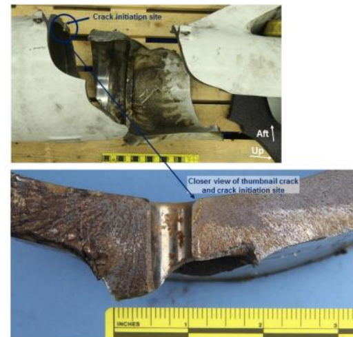
Figure 4 - Image of the air filler valve bore
