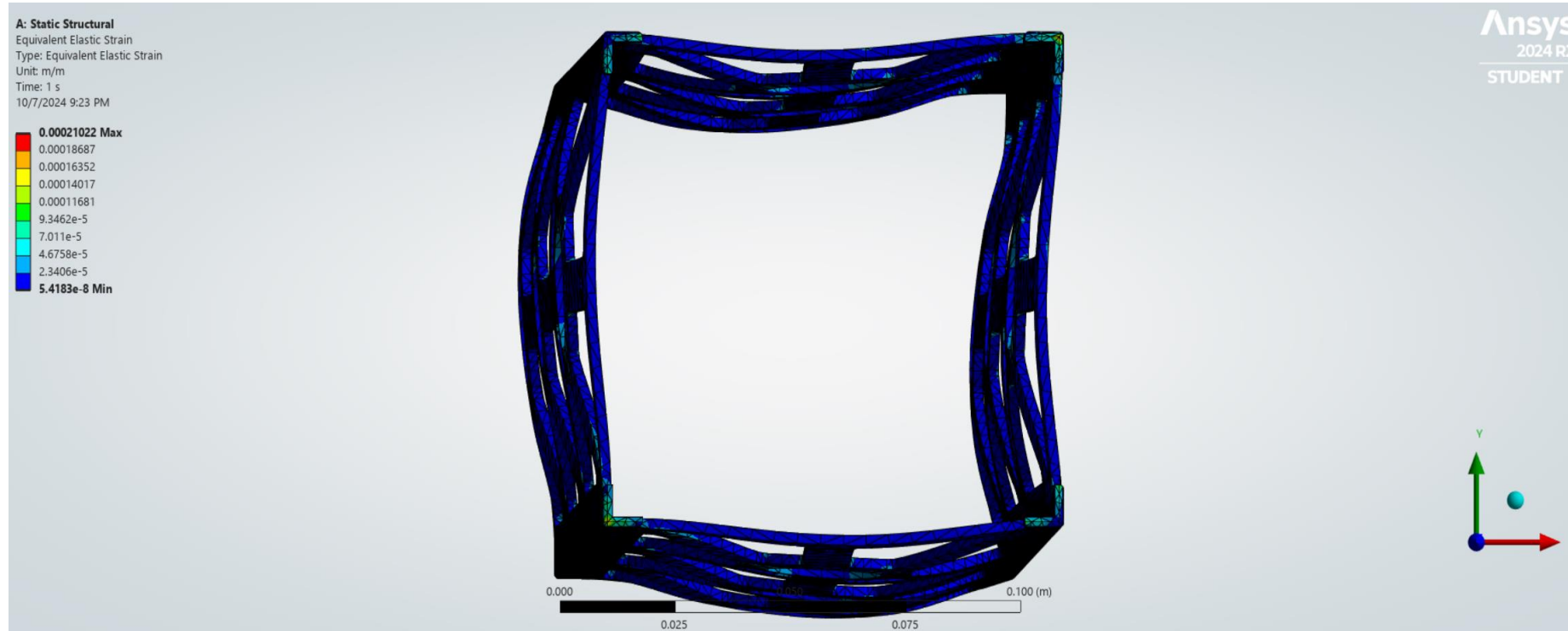
Figure 8 : Image of the equivalent elastic strain from the z-direction
