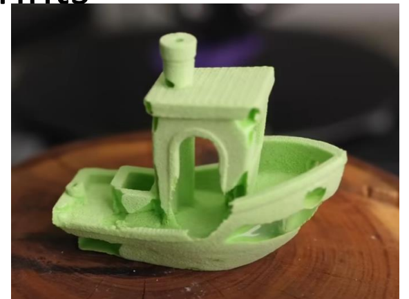
Figure 17: Example of 80% infill. Source: CNC Kitchen on YouTube
