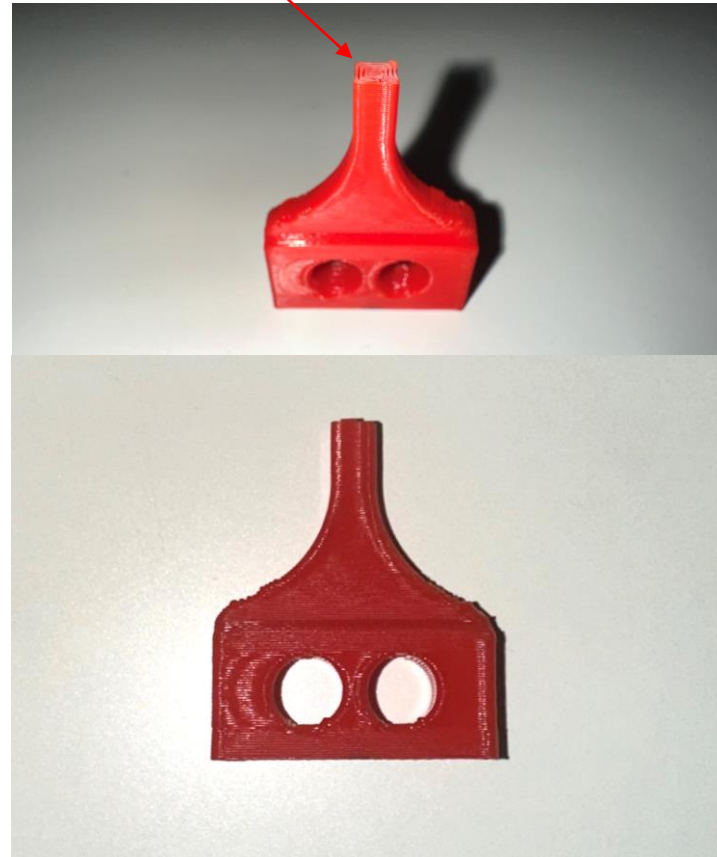
Figure 11: Although oven annealed, the layer lines didn't fuse together.
