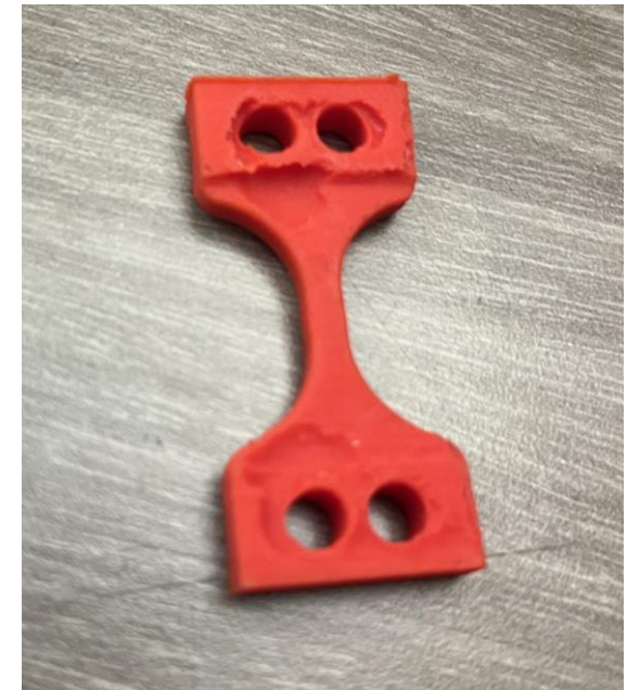
Figure 16: 180 °C salt annealed sample with cavities. Air pockets that popped as the sample was melted
