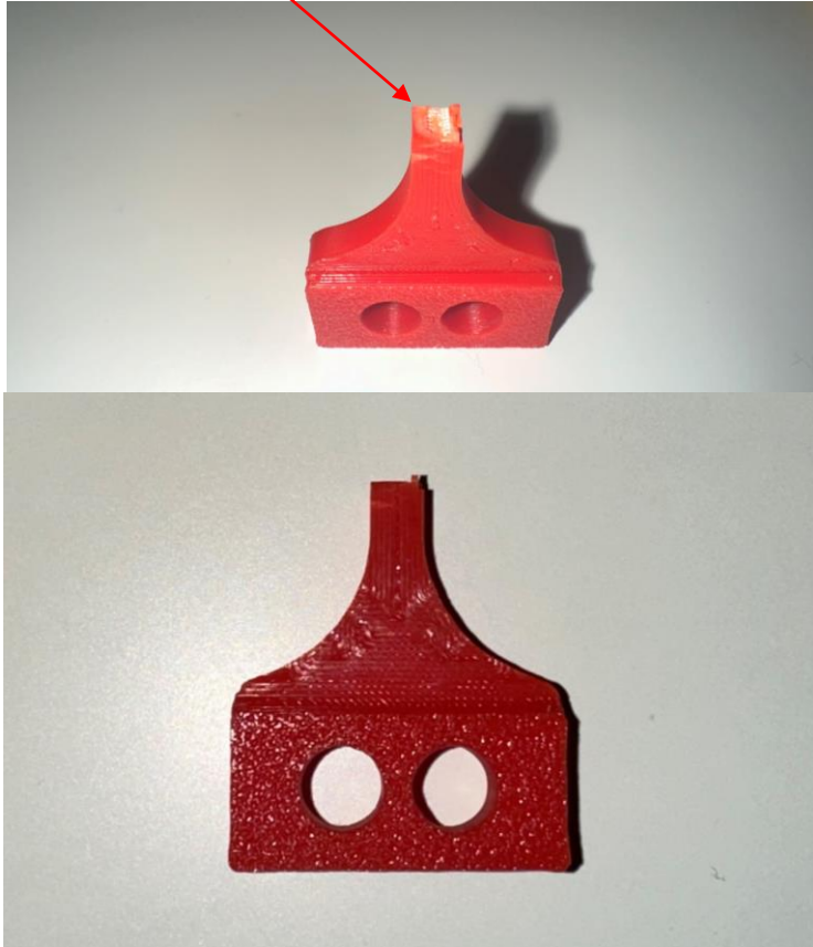
Figure 10: Breakage of horizontally printed sample.
